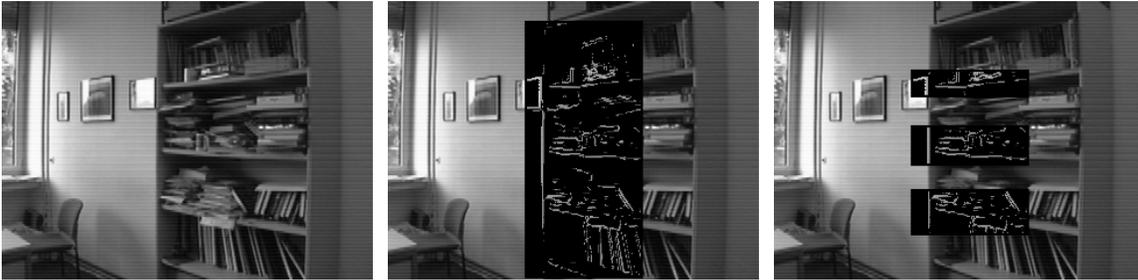
Figure 4a,b,c: Input, Canny output for 1 ROI, Canny output for 3 ROI's.
